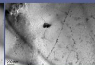
Figure 10: String of precipitates in the "B" heat treated Nb-V sample
